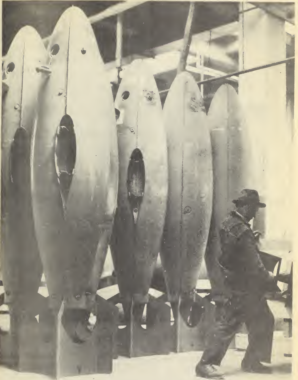
Fitting tail fins to the 165-gallon tanks to give them more bomb-like ballistic qualities.
